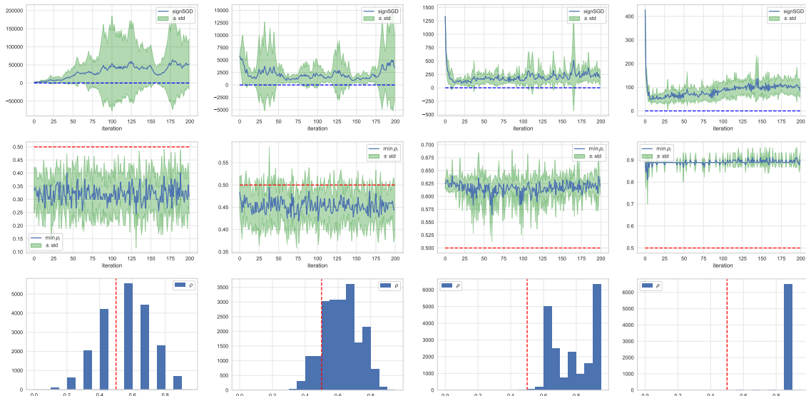
Figure 2: Performance of signSGD with constant step size ( \gamma = 0.25 ) under four different noise levels (mini-batch size 1, 2, 5, 8) using Rosenbrock function. Each column represent a separate experiment with function values, evolution of minimum success probabilities and the histogram of success probabilities throughout the iteration process. Dashed blue line in the first row is the minimum value. Dashed red lines in second and third rows are thresholds 1/2 of success probabilities. The shaded area in first and second rows shows standard deviation obtained from ten repetitions.
