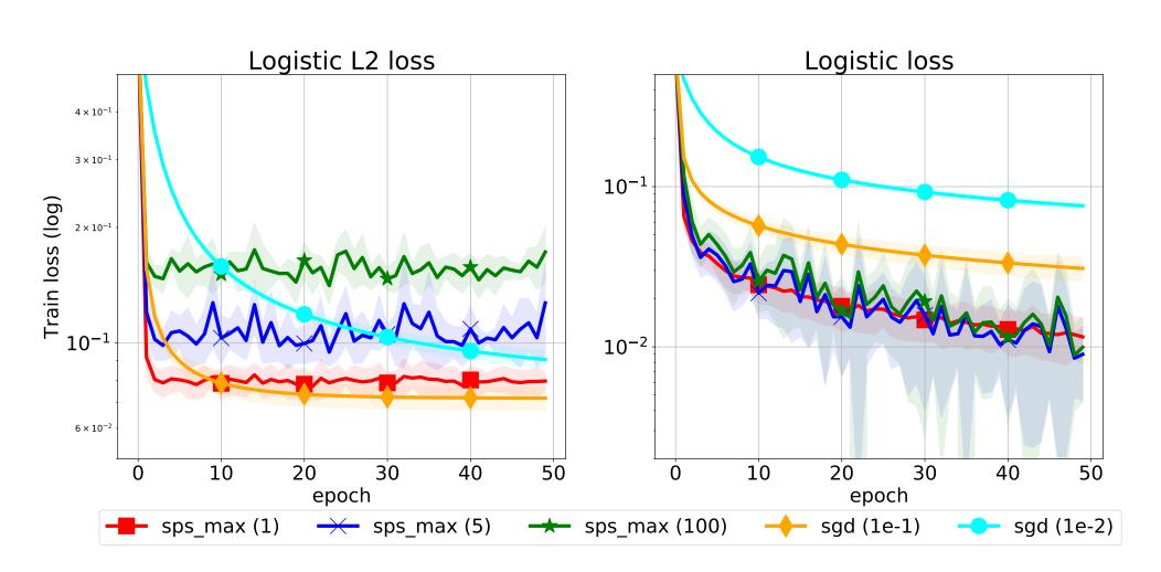
Synthetic experiment to benchmark SPS against constant step-size SGD for binary classification using the *(left)* regularized and *(right)* unregularized logistic loss.
